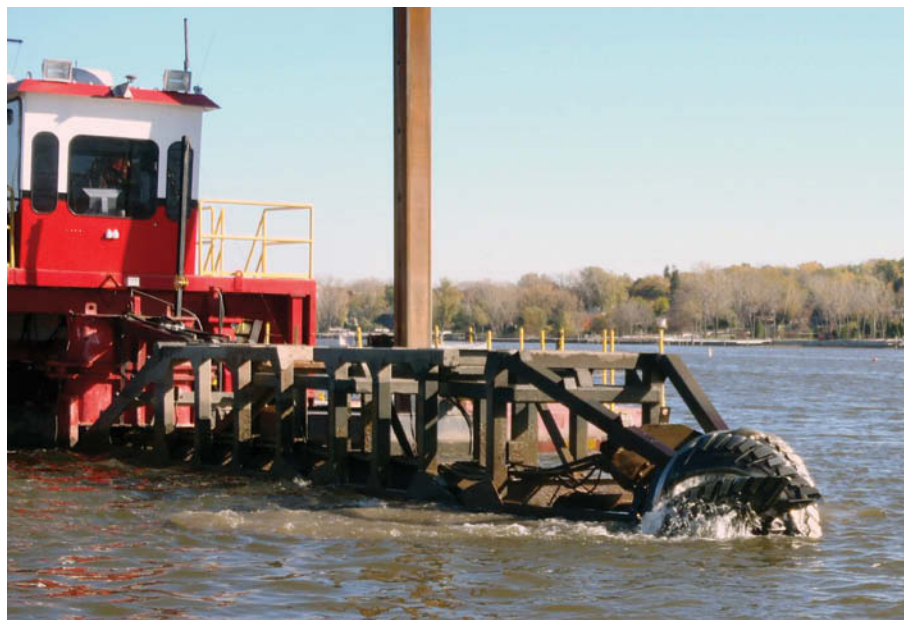
Top, the dredge operator uses satellite positioning and a digital map of the Fox River bottom to pinpoint where and how deep to dredge. Above, the 4-foot wide cutter head on the main dredge loosens contaminated sediment, while its 12-inch hose system sends the resulting slurry to the processing plant.
